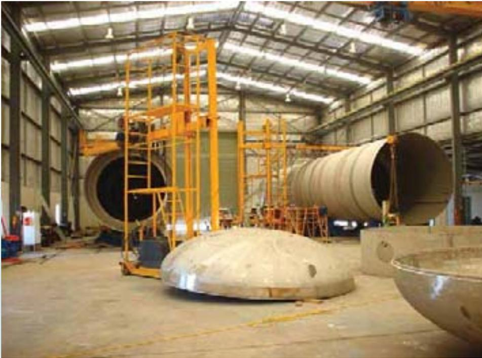
Cryeng Pty Ltd assembled two large liquid nitrogen tanks in the small fabrication shed at the AMC's common user facility for Air Liquide.
